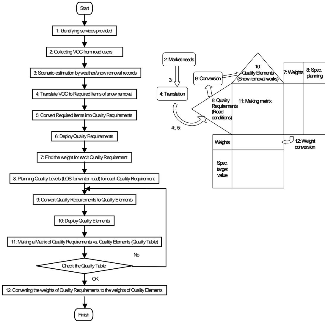
FIGURE 5 (b) Phases of QFD conducted for snow removal.
